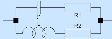
$$R = \left( \frac{1}{i\omega C} + R_1 \right) \parallel (i\omega L + R_2) = \frac{\left( \frac{1}{i\omega C} + R_1 \right) (i\omega L + R_2)}{\frac{1}{i\omega C} + R_1 + i\omega L + R_2} = \dots$$
