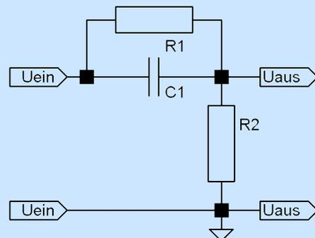
$$R = R_1 || C_1 + R_2 = \frac{R_1}{1 + i\omega C_1 R_1} + R_2.$$
